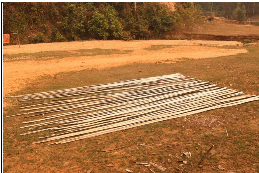
Figure 18: Split bamboo that was already soaked in water being dried
