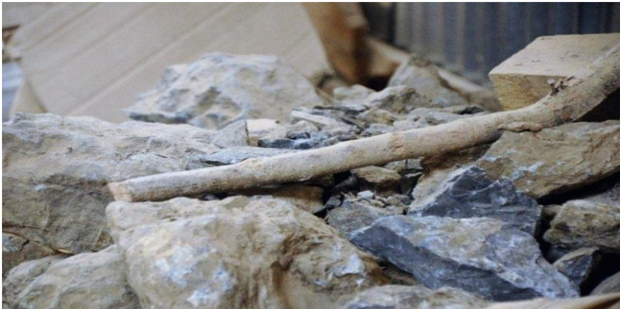
Figure 4: The sun-basked talcose serpentinite rock is broken into small pieces with the help of traditional wooden hammer.
