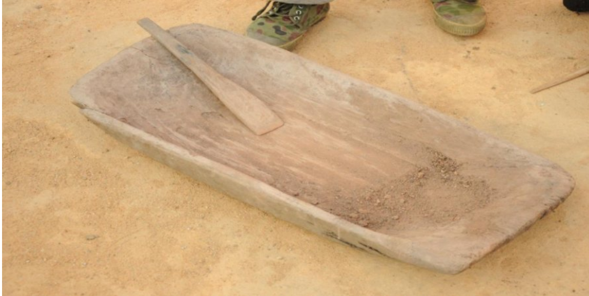
Figure 7: Likhu, a flat rectangular wooden trough that serve as a plate to mix rock powder and soil powder.
