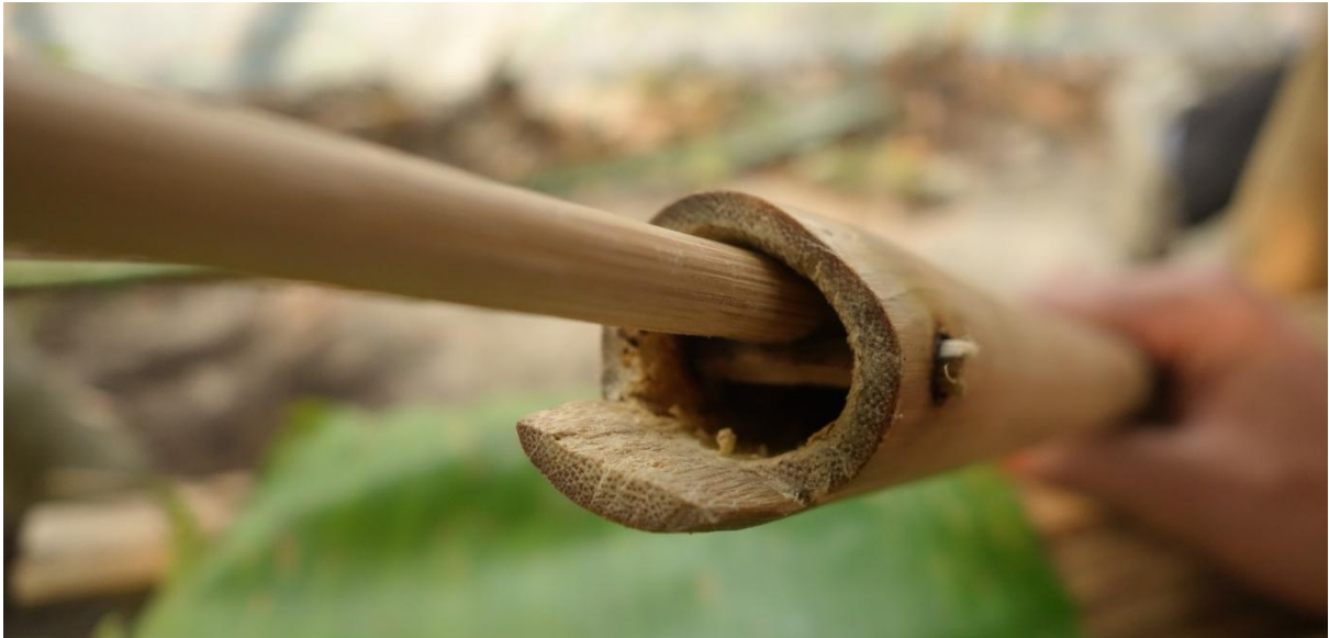
The other end of the connector goes through the lower end of the bamboo neck and is secured with a splint or by the lower node on the bamboo
