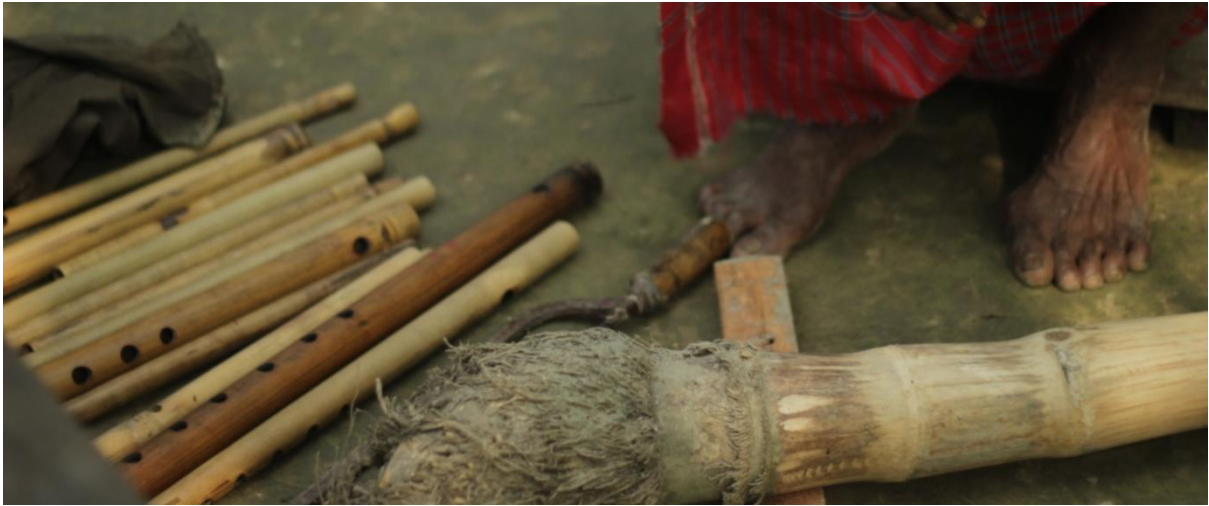
The Baro Bnaash bamboo is allowed to dry for 15-20 days before work can begin
