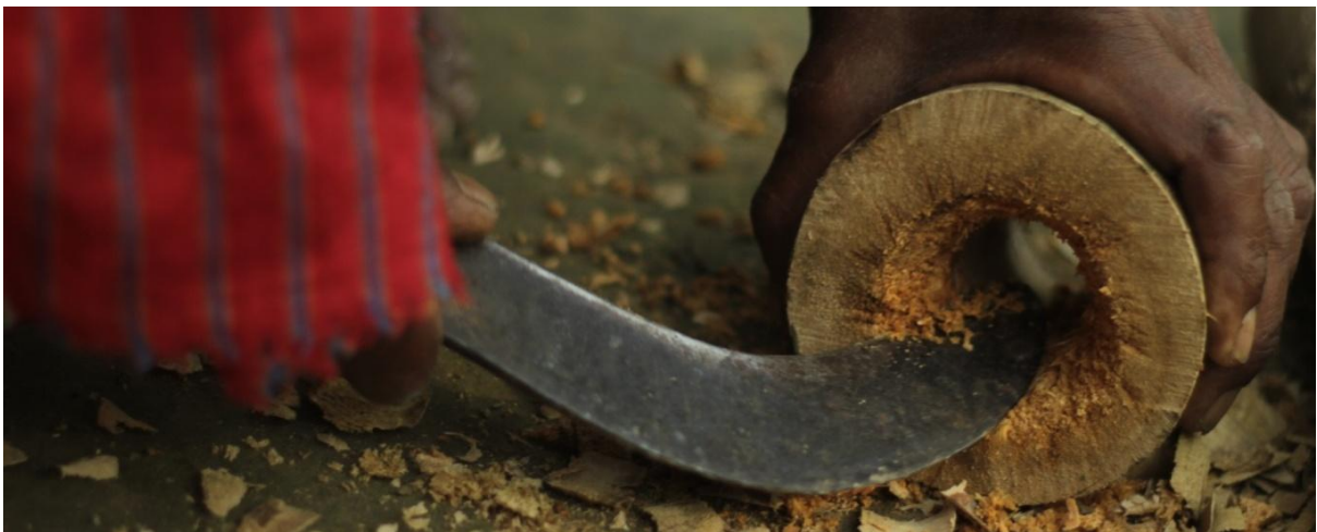
Hollowing out the sound box
