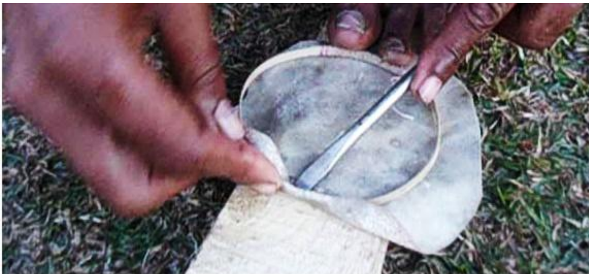
Fitting the membrane
